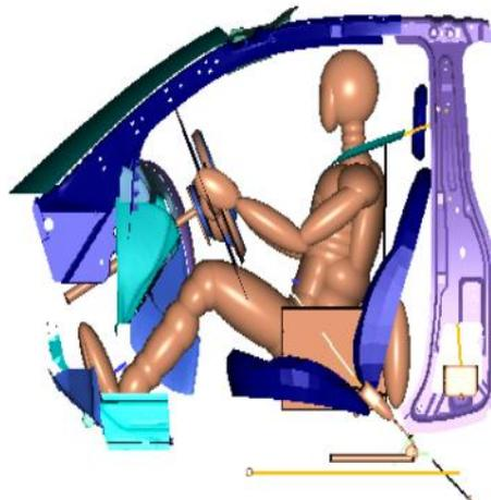
Fig. 6 Honda Accord vehicle sled model
