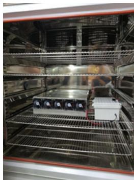
(c) Place into the temperature and humidity test chamber
