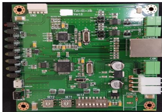
Figure 7. A pcb of the IoT module
