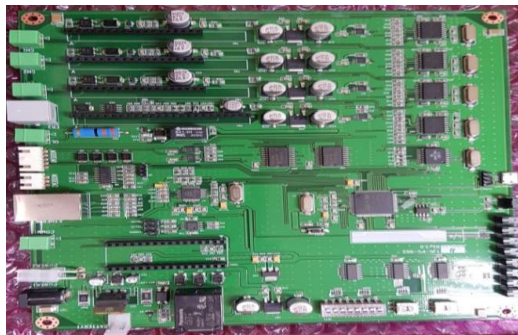
Figure 7. A PCB of the PSTN-based data collection and processing unit
