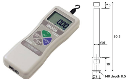
Fig. 1. Model DS2-500N (Imada, Japan) (left) and A-6 extension shaft (right), (unit=mm). ©Copyright Policy-Open Access License.
