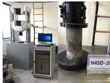
Fig. 2. UTM and Specimen Set-Up
