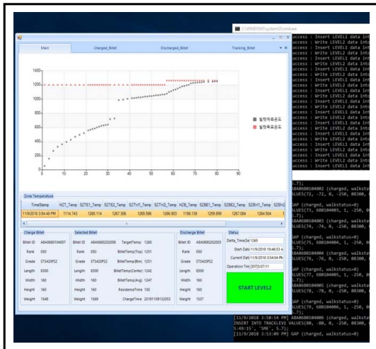
Fig. 7. Process of predicting the workpiece temperature during experiment
