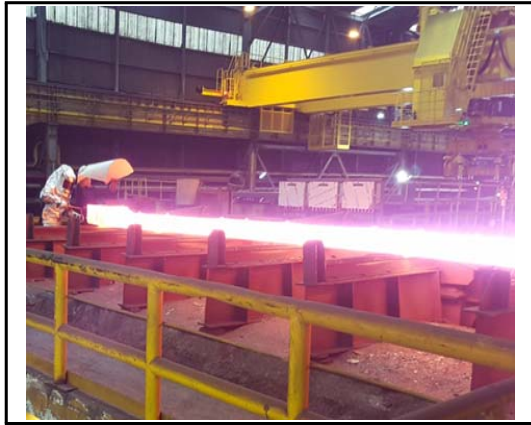
Fig. 6. Process of separating the thermal barrier box after the test workpiece is discharged
