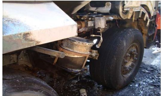
Fig. 3. Fire example by sealing fault of cylinder linear D ring part.
