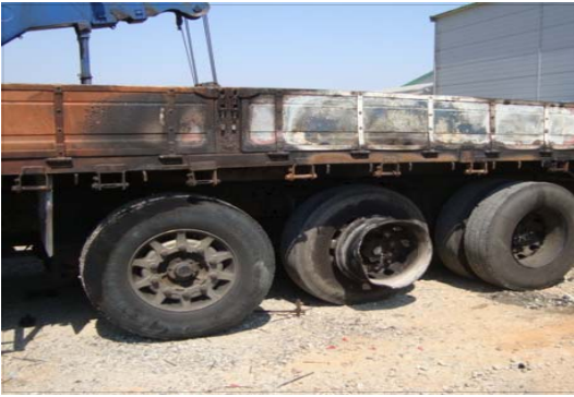
Fig. 4. Fire Example by much wear of 3 wheel brake lining.
