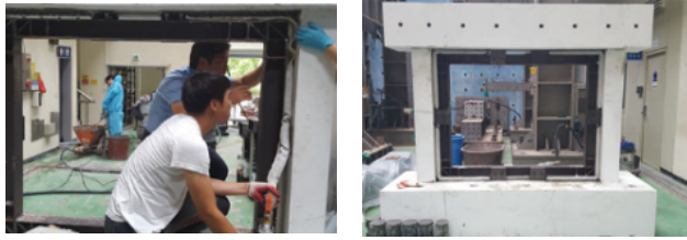
(a) Injection of expanded mortar (b) Specimens
