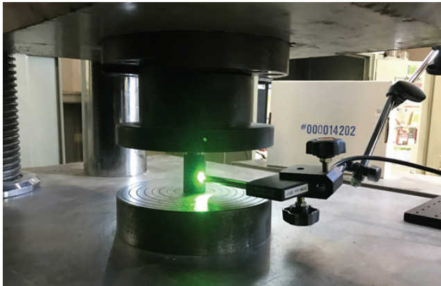
Fig. 5 Compressive Test Setup
