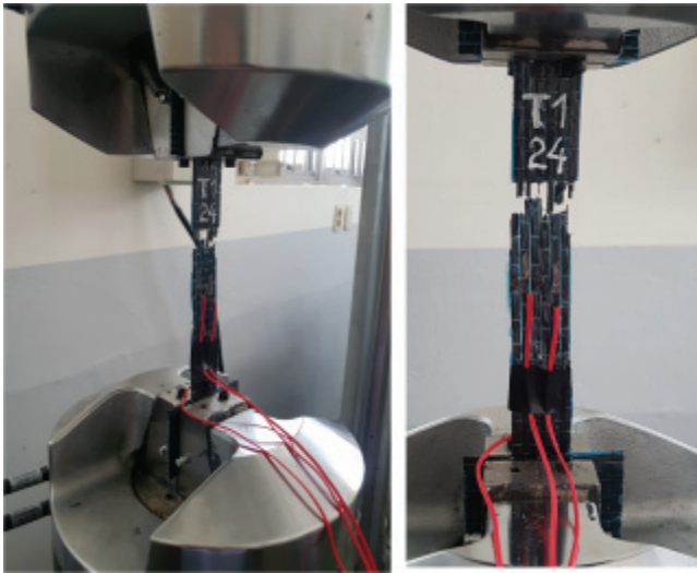
Fig. 7 Photos of T1-24 at failure
