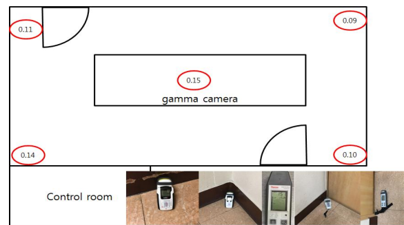
Fig. 3. Measurement of natural radiation dose rate in inspection room.
