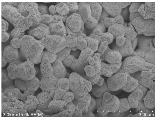
Fig. 7. SEM micrograph of alumina calcinated at 1200 °C for 5 hrs.
