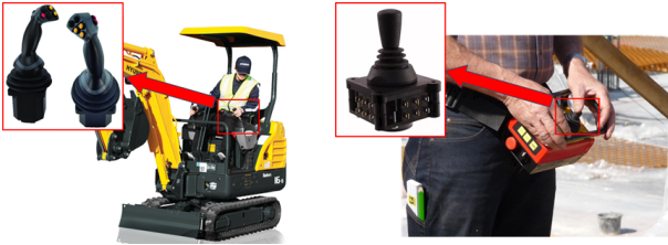
Fig. 1 Hydraulic joystick vs electronic joystick
