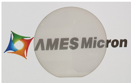
Fig. 5. GaN template grown by HVPE.
