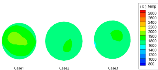
Fig. 5. Temperature contour at combustor outlet for each case
