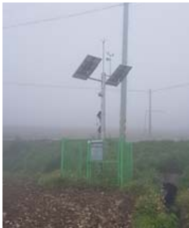
Fig. 2. The ubiquitous sensor networks established for chinese cabbage.
