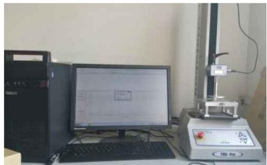
Fig. 3. TPA texture experimental device.
