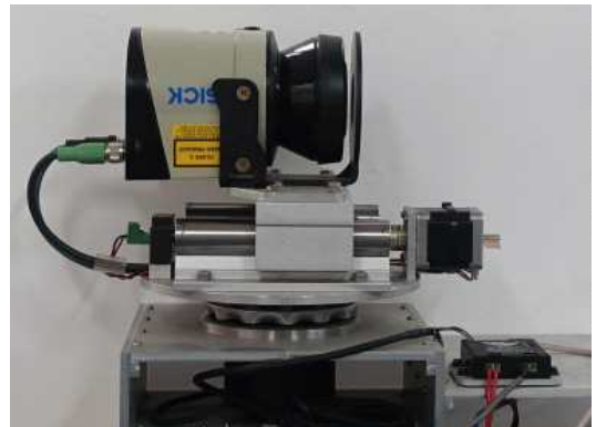
Fig. 9. Ceiling-looking 2D-LiDAR rotation module.
