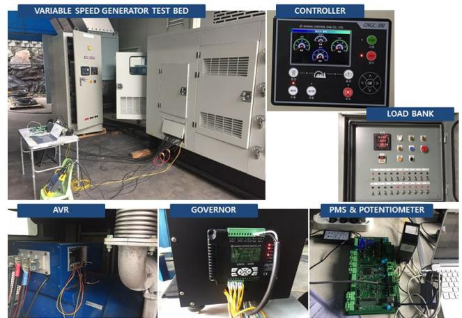
Fig. 4. Test bed for Variable speed generator test.
