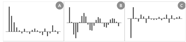
Fig. 2. Three Main Patterns of the Auto-correlation (A) The Case of Indicates that There is an Autoregressive Term in the Data, (B) The Case of Indicates that There is a Higher Order Autoregressive Term in the Data, (C) The Case of Indicates that There is a Moving Average Term in the Data
