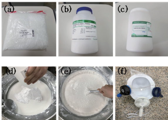
Fig. 3. (a) The paraffin wax (b) MgO (c) CaCO 3 (d) The process of mixing magnesium oxide with calcium carbonate in paraffin wax (e) MWB dissolved (f) Process of cooling and cooling PLA casting mold with MWB
