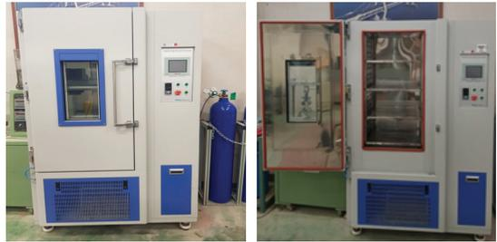
**Fig. 5** Accelerated carbonation testing equipment
