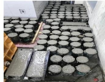
Fig. 1 Photograph of specimen making
