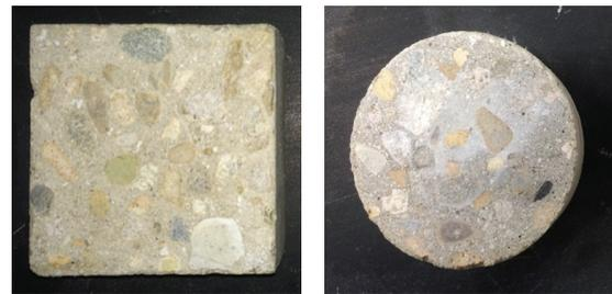
(a) A compressive load specimen (b) A tensile load specimen
