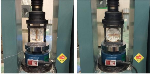
(a) Compressive load (b) Tensile load
