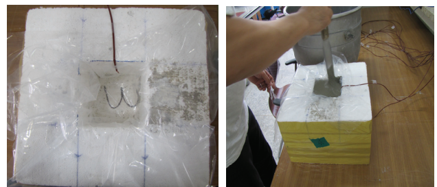
Fig. 1 Semi-adiabatic temperature rise test
