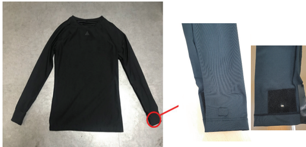
Fig. 8. Clothing for sleep apnea monitoring (Left: t-shirts, Right: Oxygen saturation wrist part)
