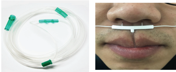
Fig. 7. Tube cartes for respiratory flow measurement
