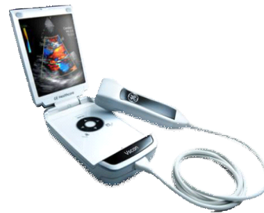
Fig. 3. GE Vscan with Dual Probe was used as a tool for measuring the position of the heart.
