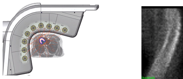
Fig. 2. Direction of each detector is directed to one place at focused SPECT.
