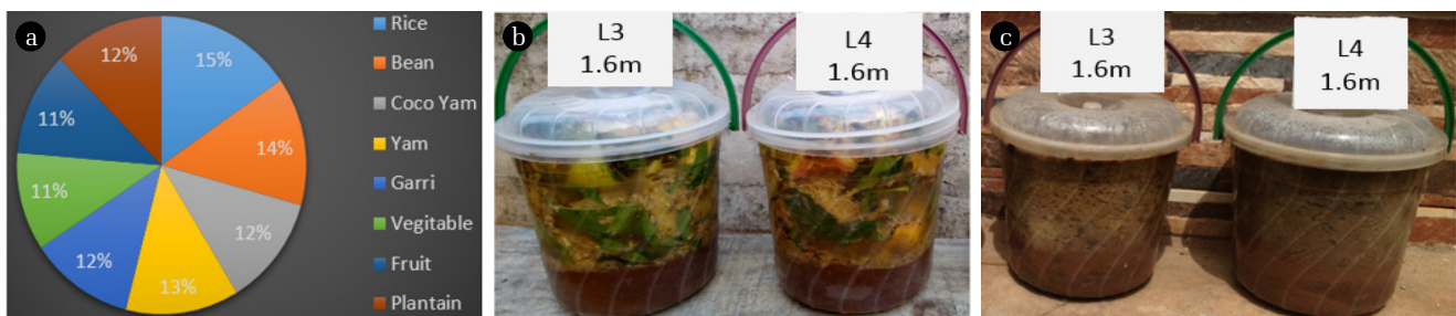
Fig. 1. Composition of food waste with soil samples. (a) Composition of food waste, (b) Mixture of food waste with soil sample, (c) Decomposed food waste with soil sample
