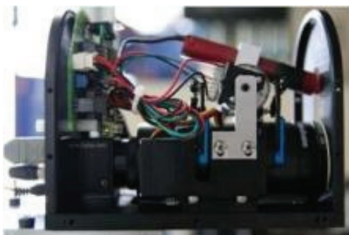
Fig. 1 Developed welding profile sensor
