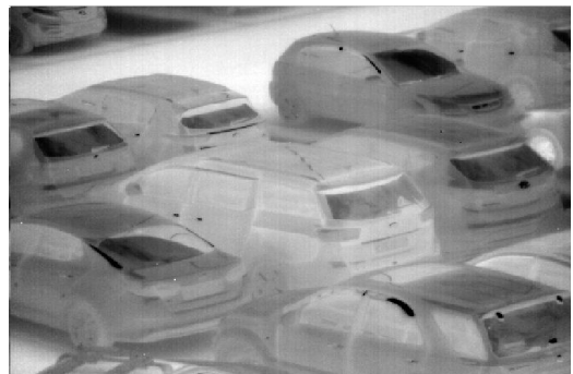
(d) FPA temperature differs 10 °C from (c)
