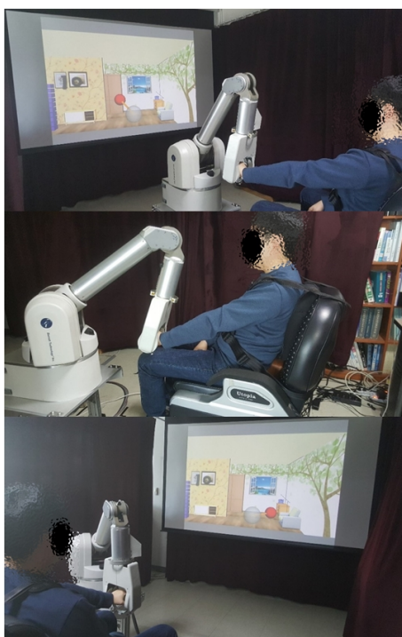
Figure 1. Setting for the robotic arm training with an assistance force program. The training test bed consisted of a Whole Arm Manipulator (WAM) and a projective display. The WAM provides a highly back-drivable motion that helps the user reach the desired sphere using point-to-point movements. A 120-inch projective display attached to the front of the test bed was used to provide suitable visual and auditory feedback to the user.
