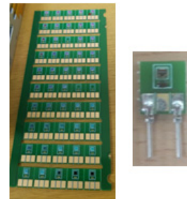
Fig. 6. Fabrication Process of the capacitive humidity sensor
