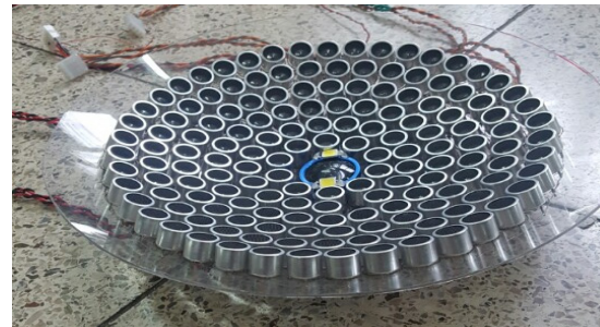
Fig. 6. Photograph of the concave ultrasound transmit module consisting of 154 ultrasound transmit elements connected in parallel, where a camera and an LED light source are placed in the center.
