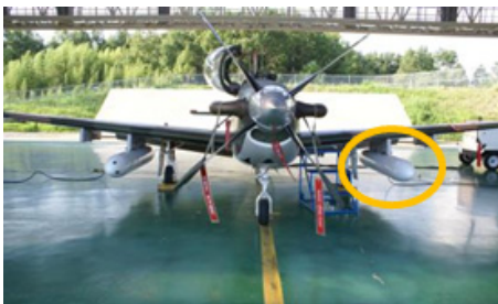
Fig. 7. Wireless POD installed on KTX-1
