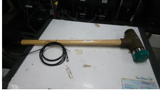
Fig. 4. Instrument equipment and impact hammer
