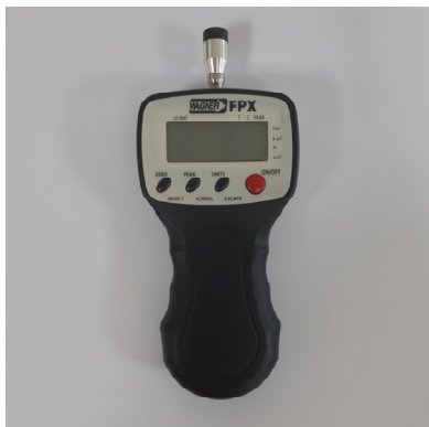
Fig. 3. FPX25 Algometer (Im-Tech, Osan, Korea).
