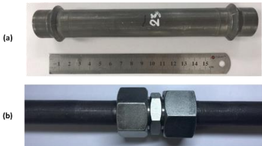
Fig. 2 Seamless pipes: (a) after compression process and (b) after connection with the bolt
