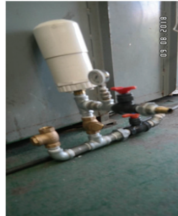
Fig. 3 Hydraulic ram pump assembled for the experiments
