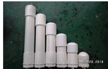
Fig. 4 Fabricated air chambers with different volumes
