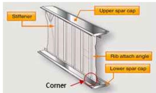
Fig. 2. Structure of I-shaped rear spar
