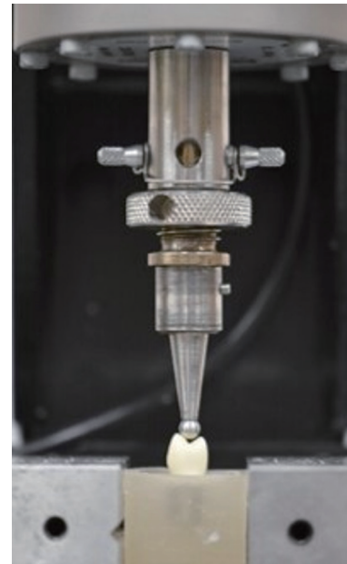
Fig. 2. Fracture strength test with the universal testing machine.
