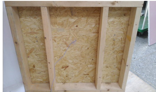
Fig. 1. Framing of wall specimen with 2 × 4 stud of 406 mm spacing.
