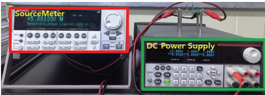
Fig. 10 Measurement setup for testing line-load regulation with precision power supply (Keithley 2230G) and source meter (Keithley SMU 2602A)
