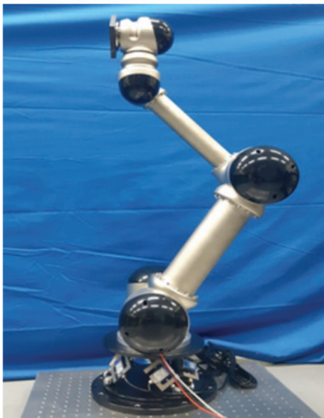
Fig. 12 Measurement experiment of a 6-DOF robot arm mounted on the base platform
