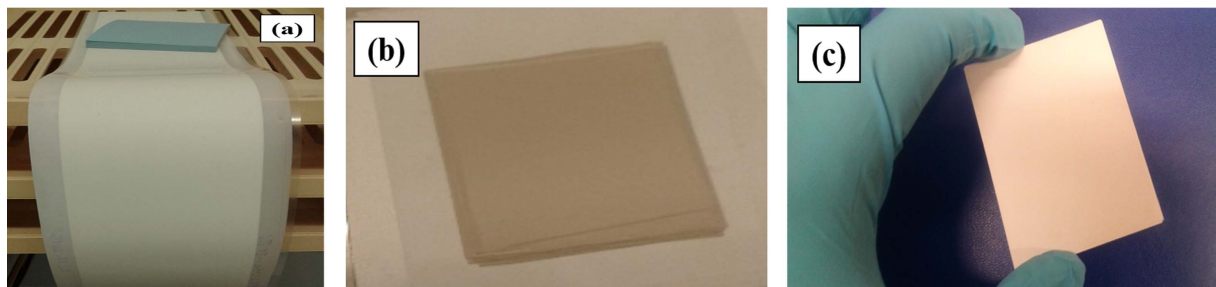
Fig. 8. Photographs of (a) cast green tape, (b) five-layer laminated multilayer substrate, and (c) substrate sintered at 900°C.
