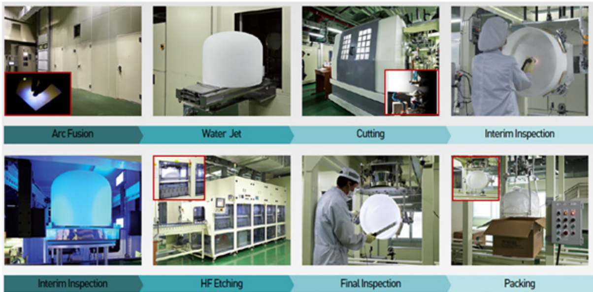
Fig. 13. Quartz crucible manufacturing process
