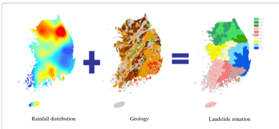
Fig. 4. Landslide prediction criteria of the Forest Service ( http://sansatai.forest.go.kr )
