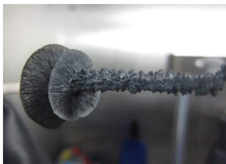
Fig. 9. (a) Chronoamperometry results obtained with an intermittent break for a two-step Zr recovery process and (b) photographic image of the Zr product.
