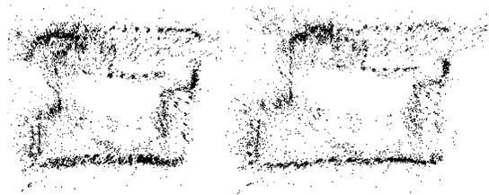
Fig. 1. (a) Map before loop closing (b) Map after loop closing.
