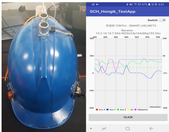
(Figure 7) Implementation of Smart Helmet and Data sensing application
