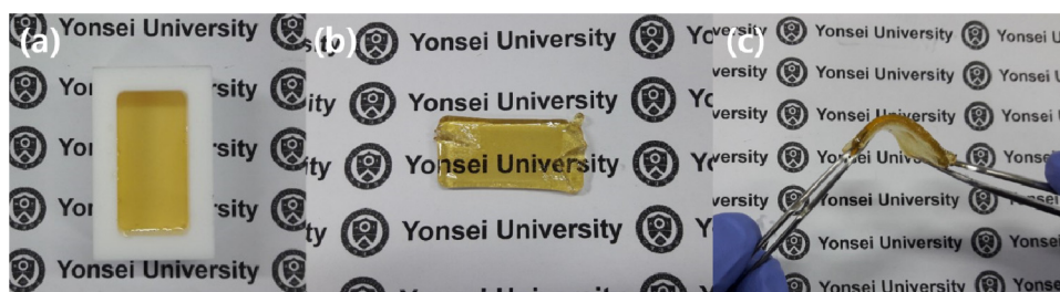
Fig. 1. Digital photos of (a) SPAN-IL solution in Teflon dish, (b) SPAN-IL electrolyte membrane after gelation process and (c) flexibility of SPAN-IL electrolyte membrane.
